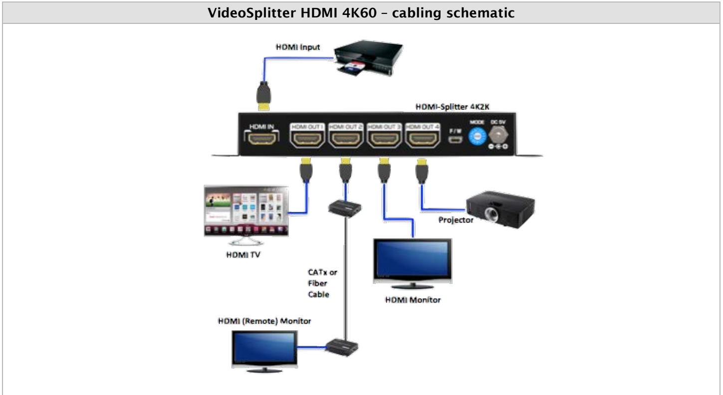
Figure 1. VideoSplitter HDMI 4K60 cabling layout diagram
