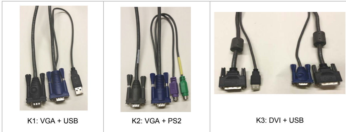
Figure 6. RackView device interface cables
