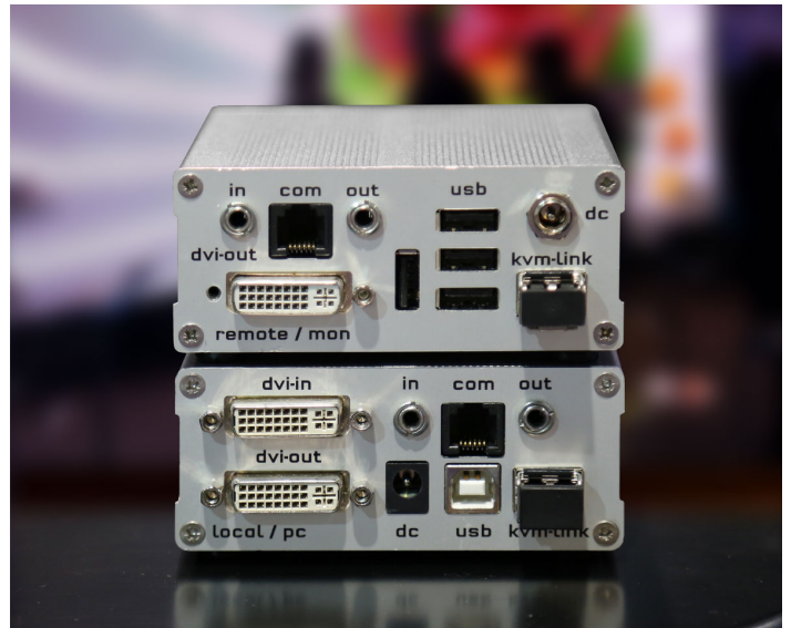
Xcion DVI Fiber Extender showing front and back panels
